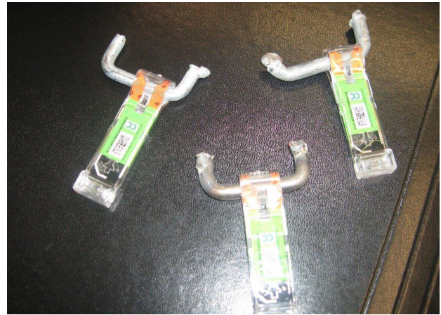
The tags are so strong that if pulled it is the metal fixing on the trolley that will often break off before the tag breaks (the average tensile strength of the tags is 120kg+).
